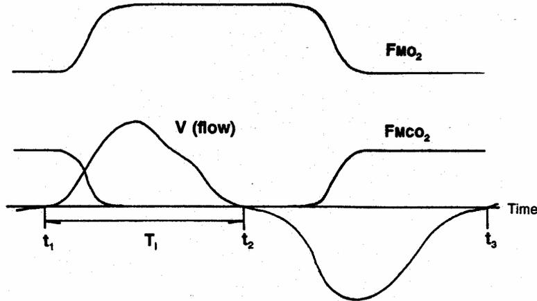
Figure 1.4-1 Illustration of a single breath  $O_2$  and  $CO_2$  concentrations and respiratory flow with definition of variables.
