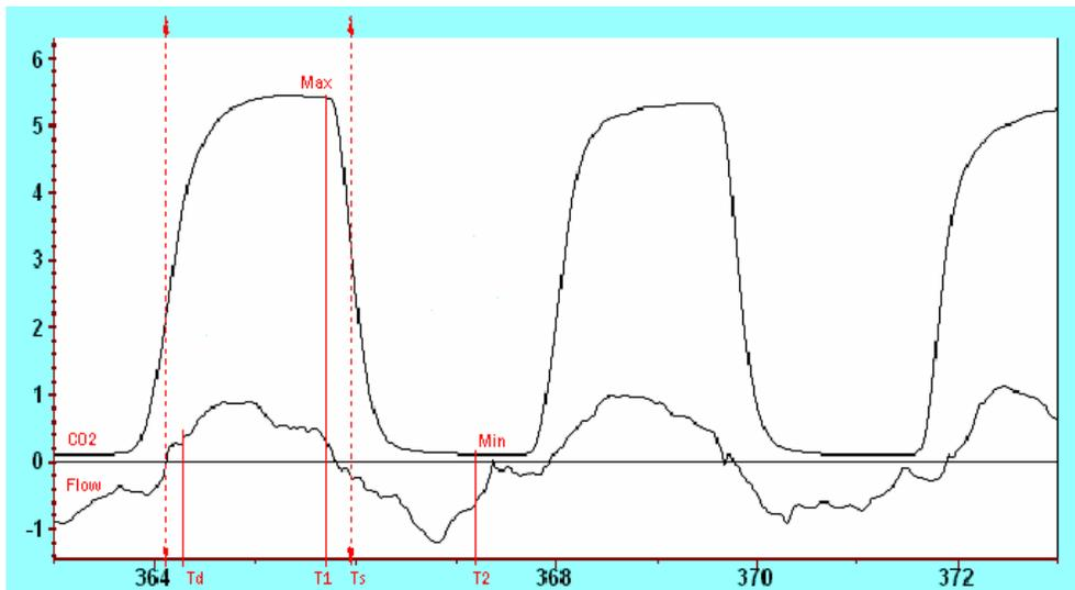
Figure 1.4.19-1 Illustration of the determination of the gas delay.
