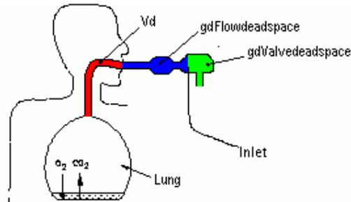
Figure 1.4.7-2 Illustration of the anatomical dead space and instrument dead spaces.
