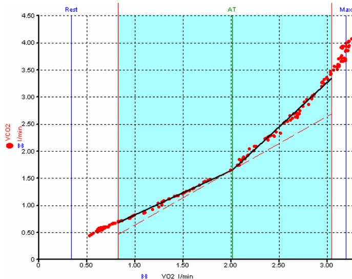
Figure 1.4.14-1 Illustration of the determination of the anaerobic threshold measured by the V-slope method.
